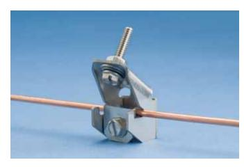
ERITECH® brand of solar bonding lugs are designed to bond the frames and mounting structures of solar photovoltaic systems in accordance with NEC® requirements. These lugs are corrosion-resistant and galvanically compatible with copper grounding conductors and aluminum photovoltaic module frames.
